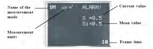
**Current value (S)** is the mercury vapor concentration in the pumped air at the current moment. (It is displayed at a repetition rate of 1 Hz and is measured in ug/m<sup>3</sup>).
